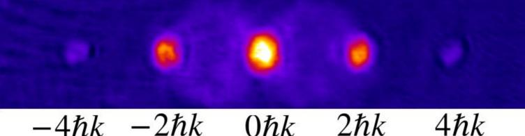
Periodic potential (optical lattice) pulsed in time  $\rightarrow$ matter wave mode split into multiple momentum components evenly spaced, p = n (2ħk)
